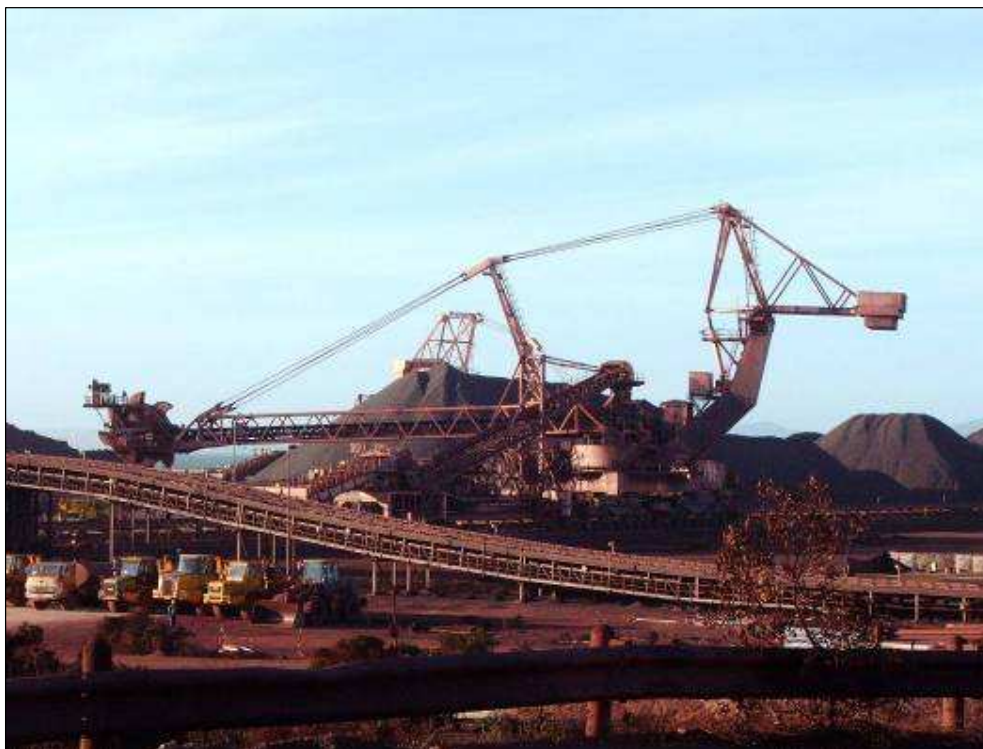
Photo Plate 2: One of three existing Stackers Reclaimers with associated conveyors
