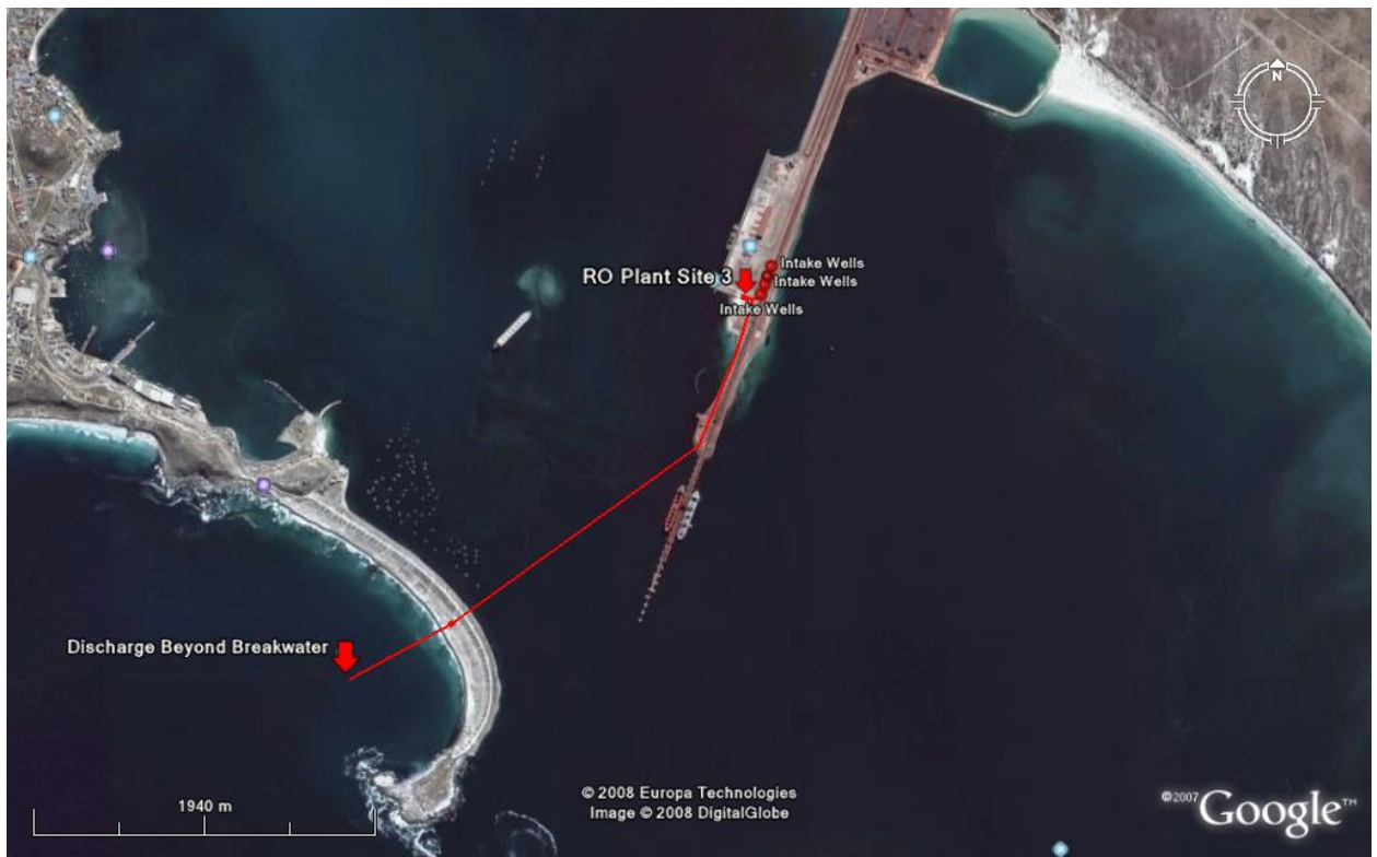
Figure 12: RO Plant Brine discharge beyond on the breakwater – Potential route for pipeline
